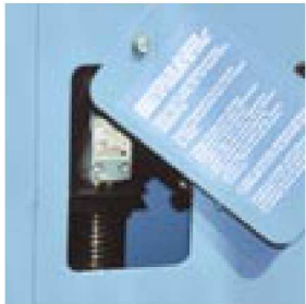
Easy inspection of the safety items through the inspection window
