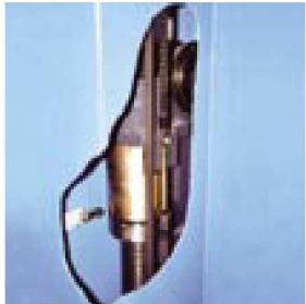
Bronze parachute nut with integrated safety nut provides a fail safe system.
