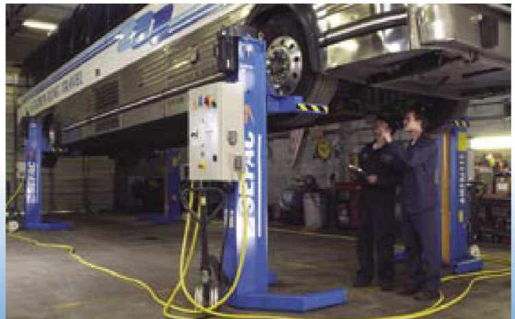
Lifts are operated by one person from any column with paired operation possible.
