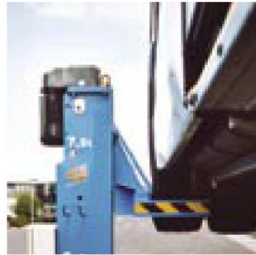
Maximum clearance between the column and the lifted vehicle combined with a much lower height than hydraulic lifts maximizes safety and eliminates vehicle clearance issues.
