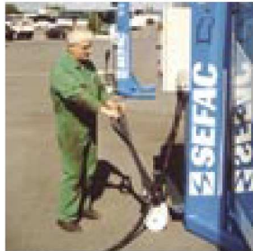
Fail safe jack handle with dead-man release.
